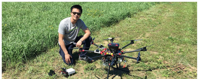
MTSU School of Agriculture Associate Professor Song Cui uses a DJI S-1000-plus drone and multispectral camera to monitor bioenergy crop production (switchgrass) at the MTSU Farm in Lascassas.
